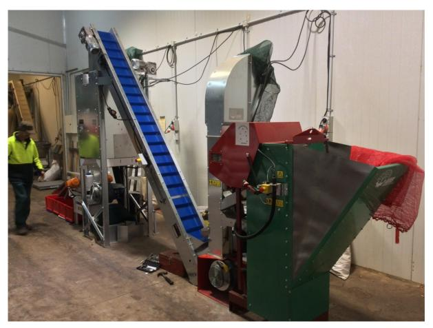
New equipment being installed at the factory – new walnut cracking plant has been purchased to improve factory efficiency and the quality of our product.
